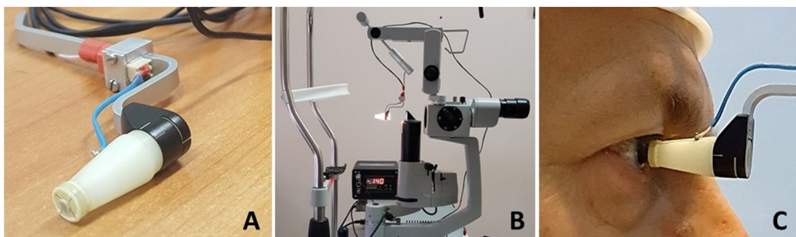
Fig. 1. The device for direct measuring of the ocular surface temperature and the HF density. The HF sensor is attached to a specially-made contact prism (A). The prism-sensor unit is attached to the Goldman tonometer's conventional prism mount. The device is attached to the slit lamp (B); The contact surface of the thermoelectric HF sensor is in contact with the human cornea during measurements (C).
